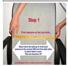
First of all, to get a proper measurement, you want to be sure all bolts are completely screwed in on the rails holding the old sling in place. Using a cloth measuring tape, be careful to measure to the nearest 1/8" as mentioned in the pictures here. If it measures between an 8th inch point always go up for the final measurement. As you choose the sling types in our store you will have drop boxes available for each dimension needed.
