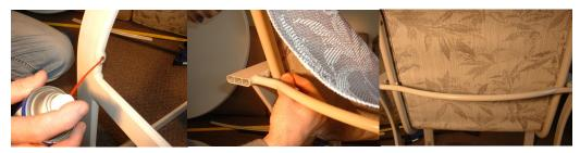
**There are some exceptions** to this as in the sling rails manufactured with a weld on one side and a long bolt on the other. Mallin, Tropitone and Carter Grandle have sling some furniture with a weld on one side and in this case you would install the sling on the welded rail first then pull the other detached rail up the other side of the sling.
