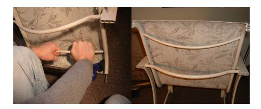
**Be careful not to over expand** the spreader bar tool but spread the rails just enough to help you replace the curved support bars in the proper holes. Keep good control of the bars as you replace them so that you do not damage the frame or the sling.
